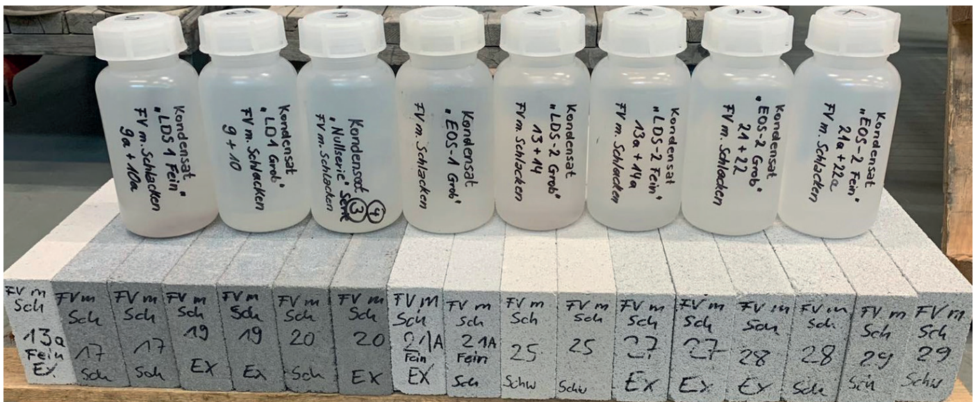
Figure 17: Some of the bricks made on a semi-technical scale for the tank leaching tests and corresponding condensates from the autoclaving process
