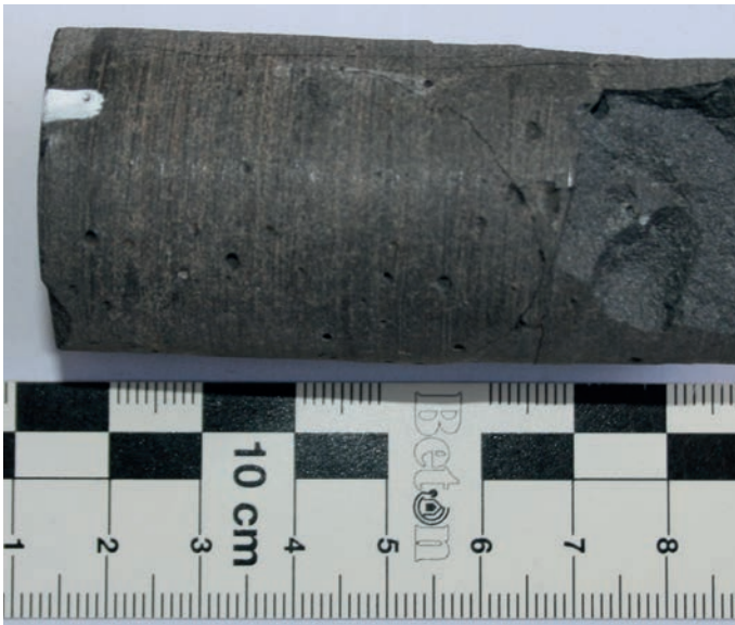
Figure 13: Damaged 5 cm drill core made from Bof-1 after the thermal expansion test
