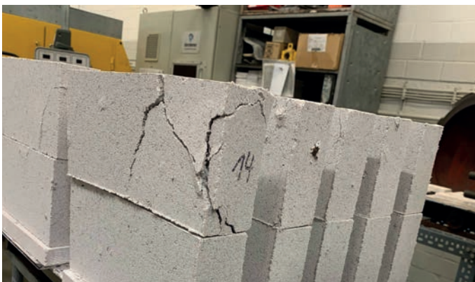
Figure 15: Damaged calcium silicate masonry units with 10 wt% Bof-2 made on a semi-technical scale
