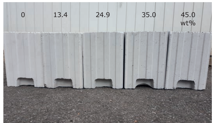
Figure 16: Damage-free calcium silicate masonry units made with COS-2 in technical scale test No. 3 with different substitution rates of the natural aggregates
